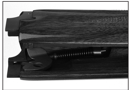
Ejection of fired shells on the Superlight Feather is selective via studs on the hammers that engage trip rods in the action body to activate the ejector sears in the gun's fore-end.
