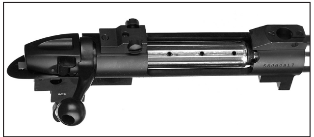
Minor points of weight reduction that add up include a semicircular relief at the front of the action's ejection port, deeper and wider bolt body flutes, hollow bolt knob and relieved bolt shroud.
